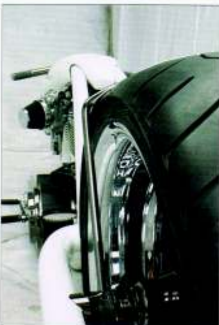
The front brake features a custom bracket to allow it to work with the radial mount
