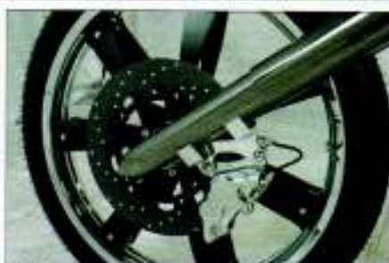
The front brake features a custom bracket to allow it to work with the radial mount
