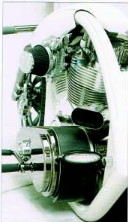
Curved license holder visually disappears behind the primary, the only clue to its existence the tail light
