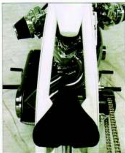
Hiding the starter, oil tank and battery creates an unusual view
